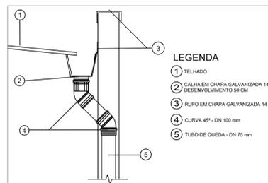
DETALHE PLUVIAL E CALHA
